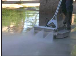
An onboard edging tool cleans close to planters, columns, and walls or use the water broom to rinse a large area
